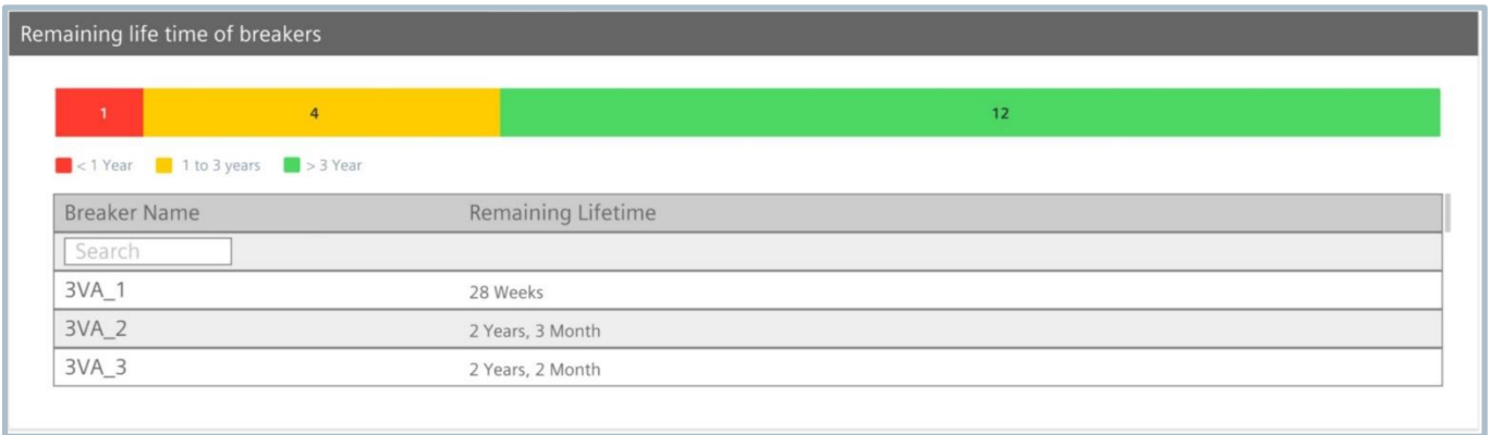
Part of a visualization example for the remaining lifetime in the power monitoring software SENTRON powermanager and the SENTRON powermind app in the MindSphere cloud.
